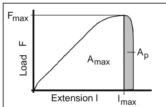
**Fig. 1:** Characteristic load–extension diagram with crack propagation energy ( $F_{\max}$  – maximum load;  $l_{\max}$  – maximum extension;  $A_{\max}$  – energy up to  $F_{\max}$ ;  $A_p$  – crack propagation energy)
