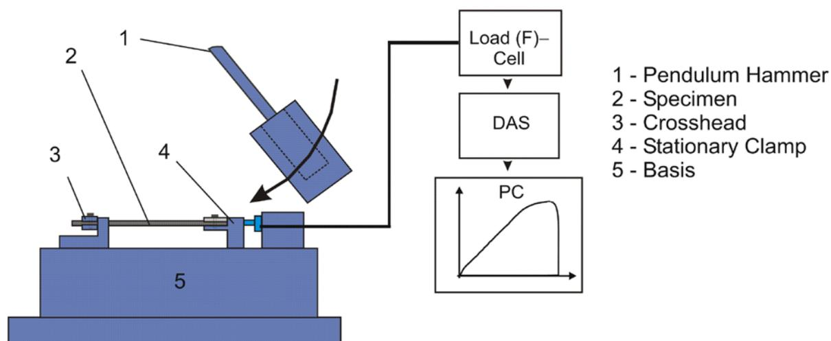
**Fig. 2:** Schematic representation of fracture mechanics testing device for performance of instrumented notched tensile-impact tests
